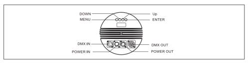
Connect the provided XLR cable to the female 3-pin XLR output of your controller and the other side to the male 3-pin XLR input of the moving head. You can chain multiple Moving head together through serial linking. The cable needed should be two core, screened cable with XLR input and output connectors. Please refer to the diagram below. DMX-512 connection with DMX terminator.
