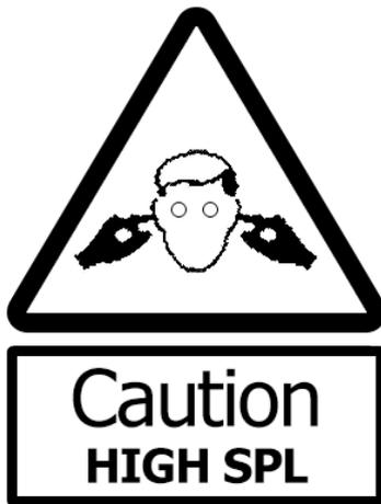
LA Series systems are capable of producing extremely high sound pressure levels and should be used with care. Hearing loss is cumulative and can result from levels above 90dB if people are exposed for a long period. Never stand close to loudspeakers driven at high levels.
