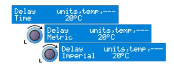
The delay units are changed in the input and output menus, with the current values being automatically converted to equivalent values.
