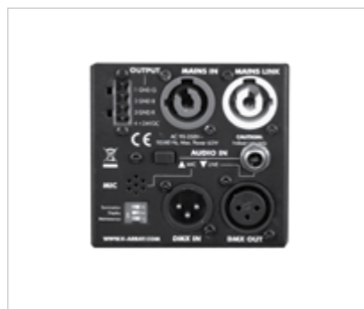
K-CTRL DMX-controlled 3-Channel power supply works as the power supply and DMX function controller for the LED component of the K-array KTL22 series of combined Speaker/Lighting fixtures. Colourmix, intensity and program operation mode can all be preset. The K-CTRL can also operate using an internal microphone for sound-to-light operation. Any settings are maintained when power is off and will return to the last setting when powered on again. A number of KTL22 series fixtures can be controlled from a single K-CTRL.
