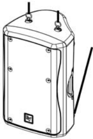
Zx5 - 2-cabinet array using 1 CB-5 cluster bracket kit
