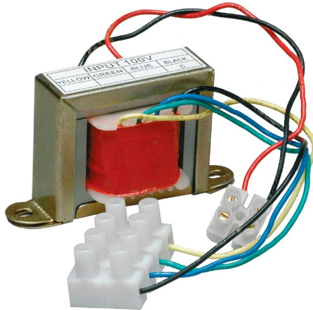
The Apart T20 is an 8 Ohm to 100 Volts transformer. By using the T20 you can change a standard 8 ohm loudspeaker into a 100 Volts loudspeaker.
