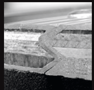
To reach the desired strength, the edge of the wood was finished right up to the profile. The used wood is 3/8" multiplex.
